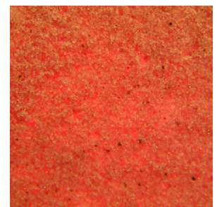
Microscopic view of Lactose and Dyed Corn Starch at 60 seconds (40x magnitude)
