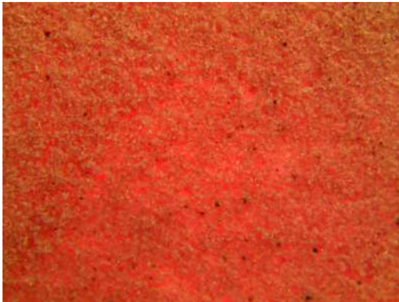
Microscopic view of Lactose and Dyed Corn Starch at 60 seconds (40x magnitude)
